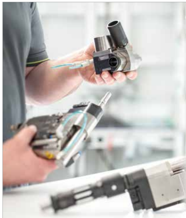
Left: The Quick Change System allows a quick changeover of locking systems.
