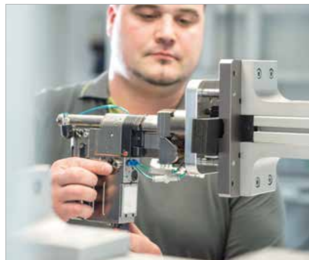
Below: Drilling tests according to customer specifications using a supplied cutting tool and supplied drilling material.
