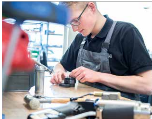
Below: Assembly of a Quick Index Adapter at an L.ADU pneumatic.
