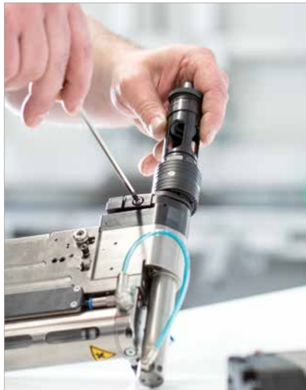
Left: Assembly of a Quick Change Indexing adapter to an L.ADU pneumatic.
